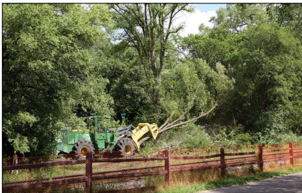
The John Deere Feller Buncher machine removing trees and underbrush at the Kenilworth Trail and Cedar Lake Parkway.
