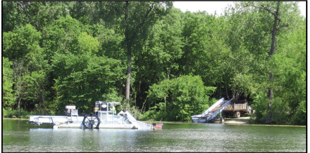
Peter Lane, Park Board mobile equipment operator, readies the harvester for its forays against Eurasian water-milfoil and curly-leaf pondweed. The harvester is moored at South Point near the west shore of Cedar Lake. The conveyor belt can be seen on shore. (Photo and caption: Michael Wilson.)
