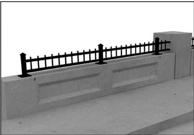
Close-up view of new 3' 6"-high railings, designed to meet current crash-worthiness standards.
